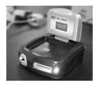
The QLCA represents a shift in the design of POC analyzers. The QLCA is a small, portable, stand-alone and completely automated point-of-care immunoassay analyzer. The QLCA has successfully miniaturized lab test technology, and combined it with a simplified mechanical design and proprietary triggering mechanism.
